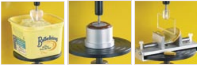
Penetrometry Back Extrusion Snap Testing
